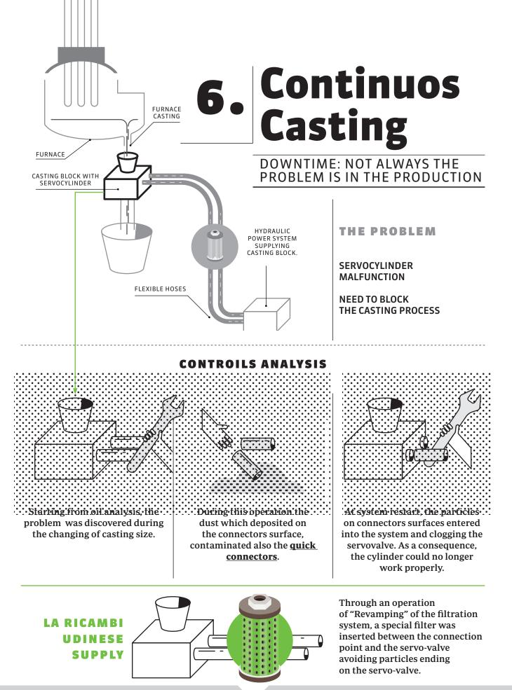
WITH THIS SOLUTION, THE DUST THAT COULD SETTLE ON CONNECTORS AND THAT COULD BE DRAGGED INSIDE THE SERVO-VALVE, IS SHUT OFF BY THE FILTER. THANKS TO THIS SYSTEM, ALSO THE STOP OF THE CASTING WAS ELIMINATED.
